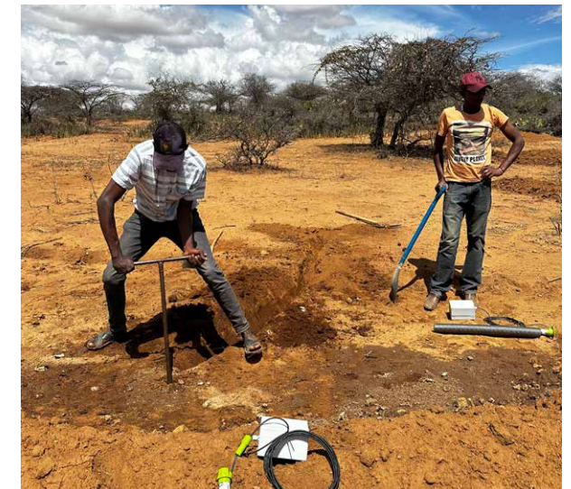
Community members in action: Installing soil moisture and temperature probes Photo: Marcel Wälti
